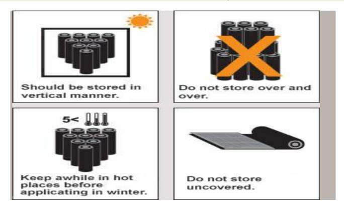
The rolls of bituminous membranes should be stored in vertical manner. Additionally during the transportation they should be placed vertically.
